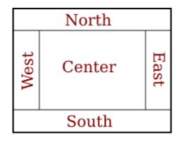
Note that a border layout can contain fewer than five components, so that not all five of the possible positions need to be filled. It would be very unusual, however, to have no center component.
