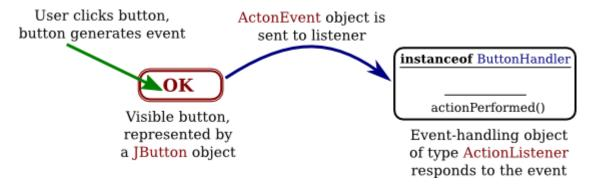
As an example, consider the OK button in the sample program. When the user clicks the button, an event is generated. This event is represented by an object belonging to the class *ActionEvent*. The event that is generated is associated with the button; we say that the button is the source of the event. The listener object in this case is an object belonging to the class *ButtonHandler*, which is defined as a nested class inside *HelloWorldGUI2*:
